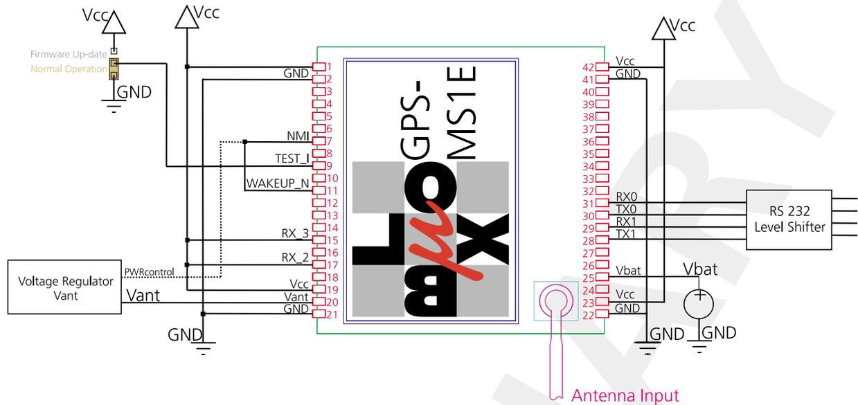
**Figure 3: External wiring (Continuous and TPM mode)**
